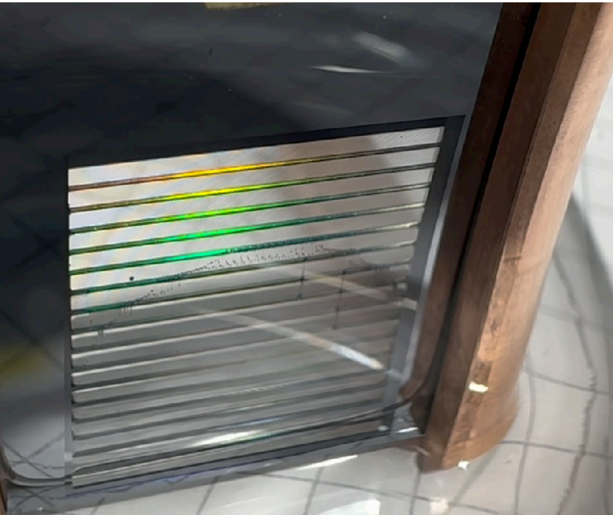
Capillary effect (with acetone)
