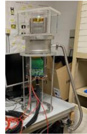
Lab test of High voltage stability under vacuum (bottom)
