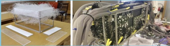
SFGD prototype test beam & mechanical tests of the box
