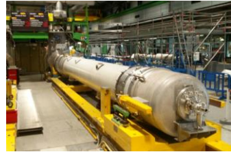
HL-LHC 12 T Nb 3 Sn quadrupole
