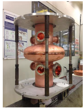
400 MHz 1-, 2- & 4-cell Nb/Cu , 4.5 K
