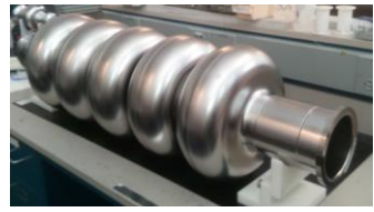
800 MHz 5-cell Nb prototype / JLAB, 2 K
