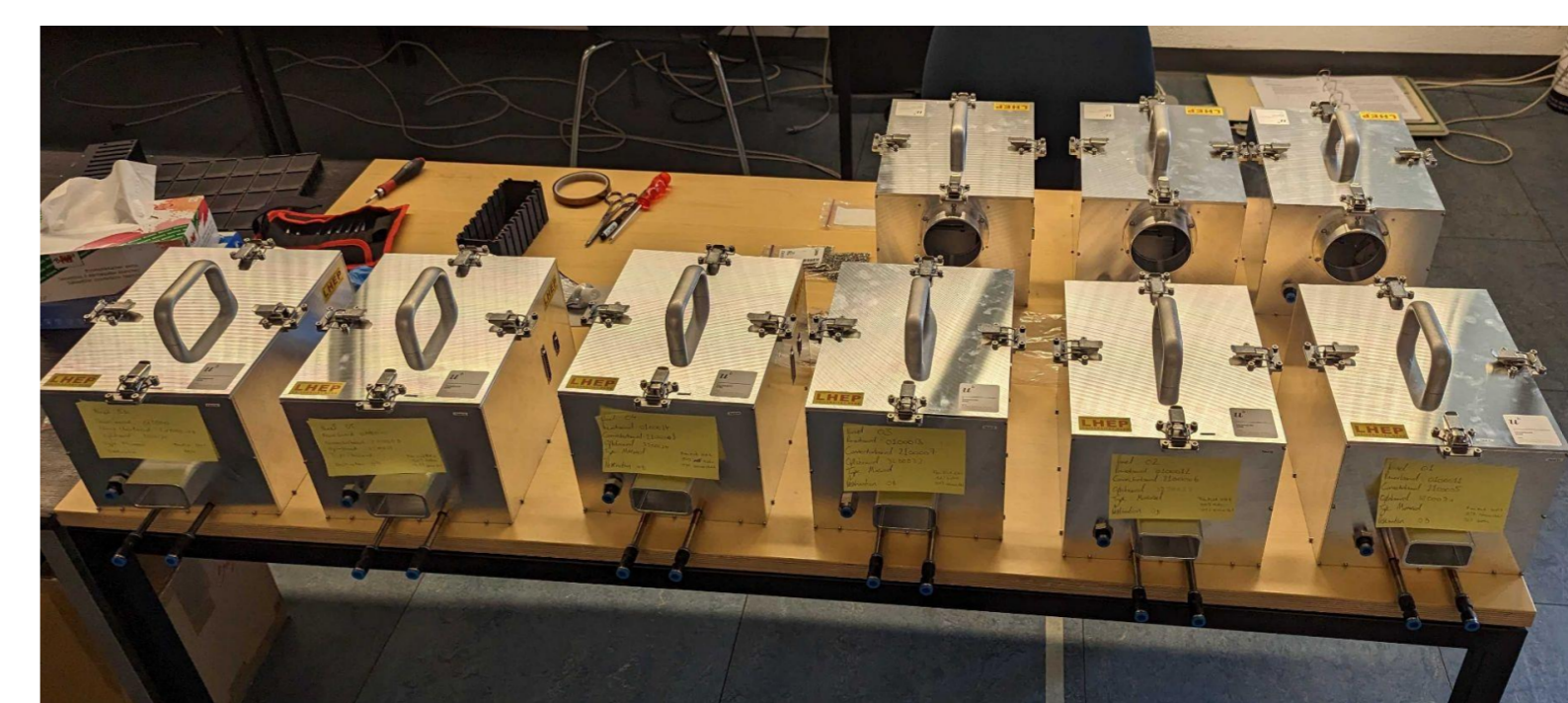
FIG. 10: Single-box Optopanel for LLS, each containing one Optoboard.
