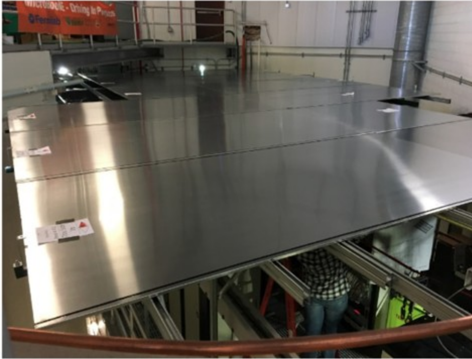
Cosmic-ray tagger (CRT) system ~200 m 2
