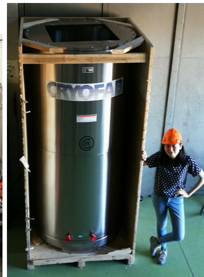
Single Module Cryostat
