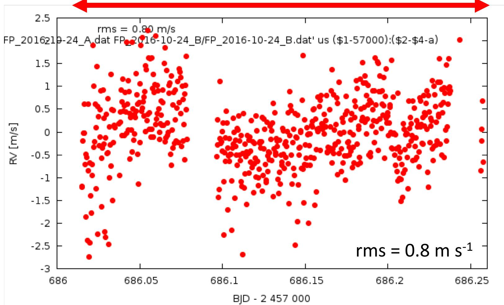
Stability of  $\sim \text{m s}^{-1}$  over short timescale demonstrated with FP light
