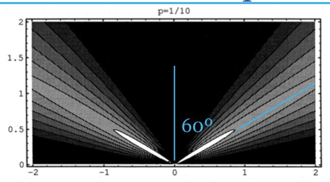
Twisting/winding causes field lines to open radially
