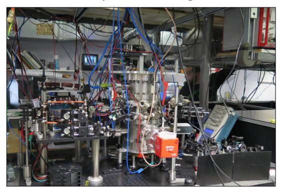
Experiment rotated by 90 degrees from the Berkeley experiment, so that no sensitivity to Earth's gravity
