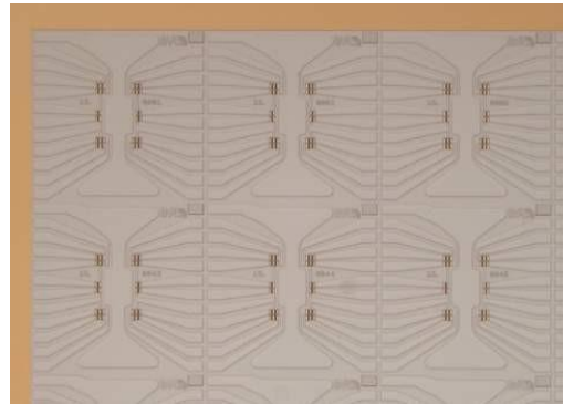
Figure 20- Optical image after lift-off. No sacrificial layer on source, drain and channel.
