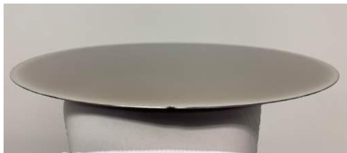
Figure 19- Picture of the wafer after sacrificial layer deposition.
