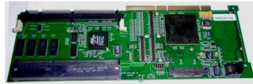
IOP card with on board CPU, 3 PCI buses Altera FPGA
