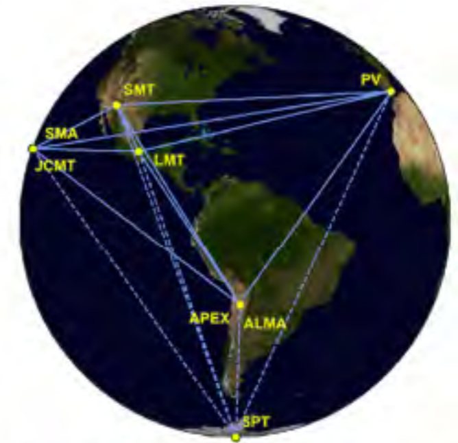
Figure 1. Light stations of the EHT 2017 campaign over six geographic locations as viewed from the equatorial plane. Solid baselines represent mutual visibility on M87* ( \pm 12^\circ declination). The dashed baselines were used for the calibration source 3C279 (see Papers III and IV).
