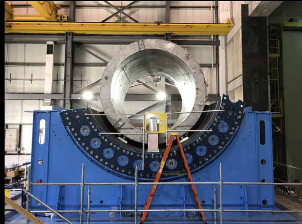
Magnet landed in the partially assembled flux return and outer HCAL (in 2021)
