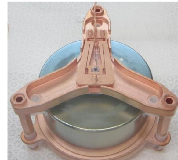
Array components and passive shielding fabricated from ultra-pure materials with extremely low radio-isotope content
