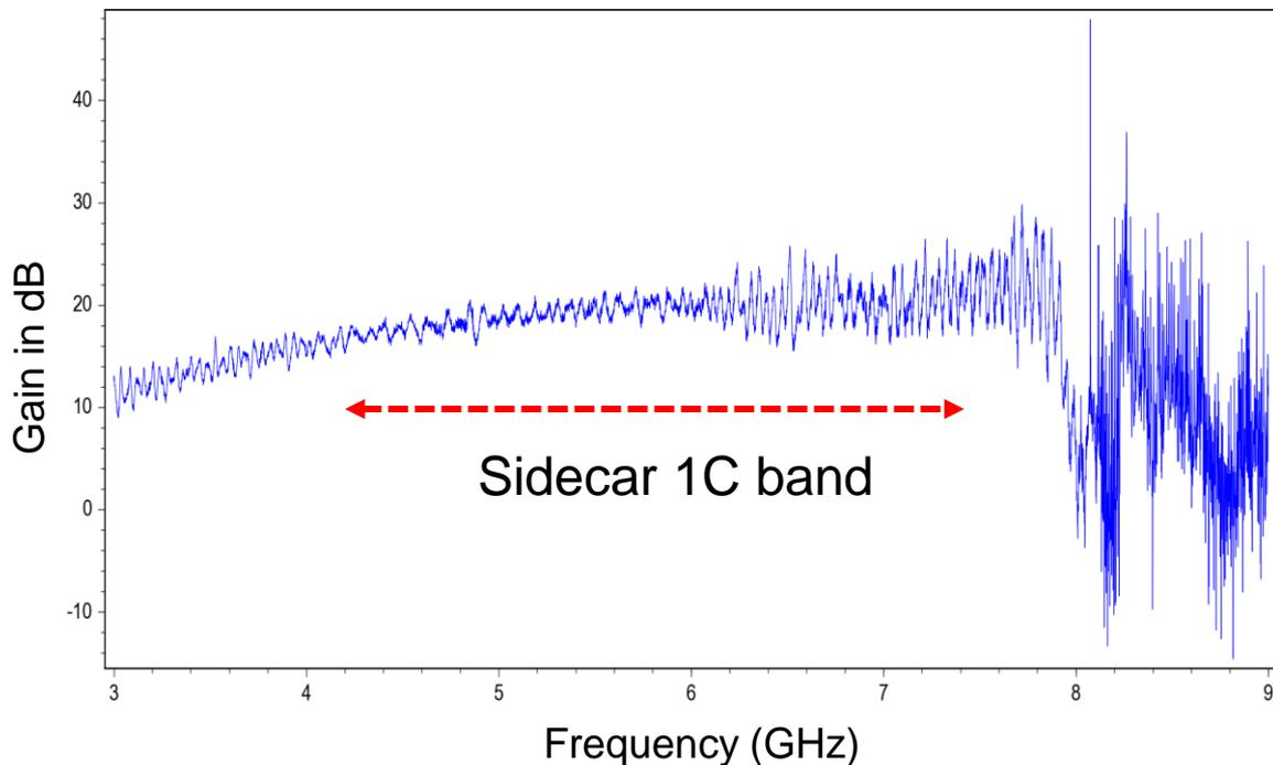
Signal to Noise Improvement (pump on vs pump off)
