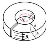
Toroidal geometry for zero-field detection
