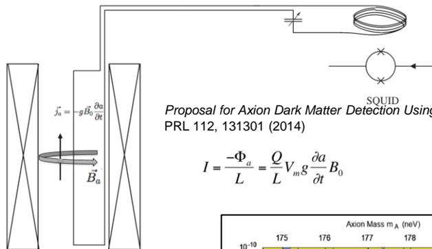
Proposal for Axion Dark Matter Detection Using an LC Circuit
