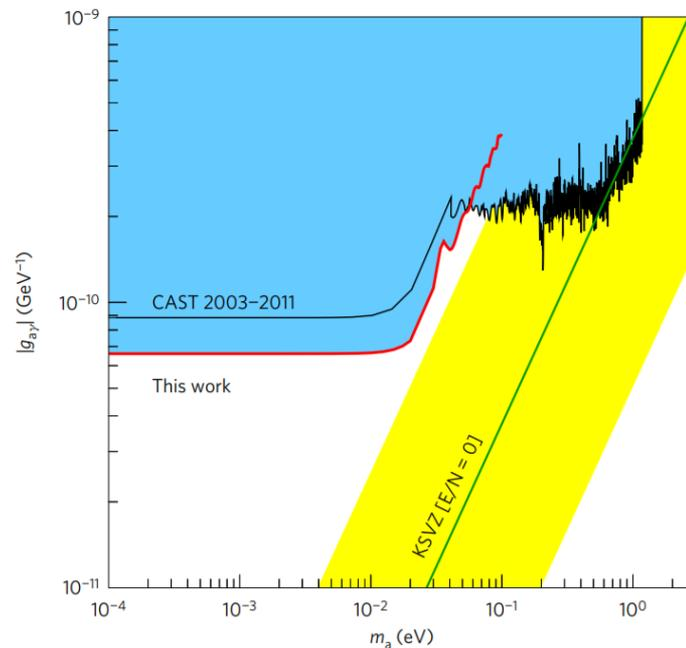
CAST best limits for relatively high mass ( $\sim \text{eV}$ ) axions
