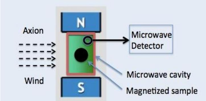
The effective magnetic field associated with the axion wind
