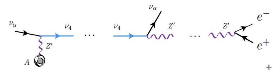
Mz should be light (< 60 MeV) so that the electron pair is collimated and can "fake" an electron-neutrino ring
