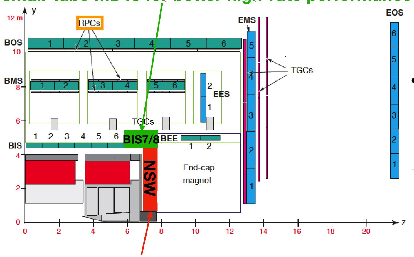
Thin-gap chambers (TGC) provide triggering in the endcap
