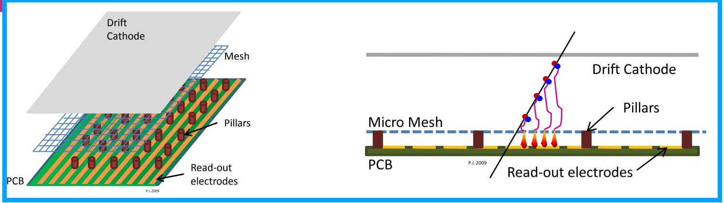
New for Run-3: upgrade of the Small Wheels to handle higher luminosities with better spatial resolution and improved triggering
