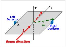
The beam  $(\uparrow\downarrow)$  and target  $(\pm)$  single spin asymmetries are concurrently measured using  $0.5 < T_R < 10$  MeV recoil protons.
