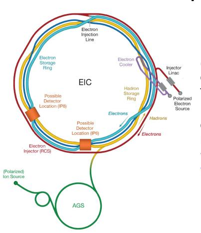
High energy, 40-275 GeV polarized proton and helion (<sup>3</sup>He<sup>↑</sup>) beams are planned at the future Electron Ion Collider.
