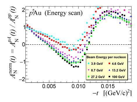
In the Au beam measurements at HJET ( $\Delta \gtrsim 4$  MeV,  $3.8 < E_{\rm beam} < 100$  GeV/n), no evidence of the breakup fraction in the elastic data was found.
