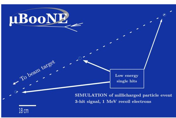
Isolated hits with argon electron in a straight line. Favors low-energy hits.
