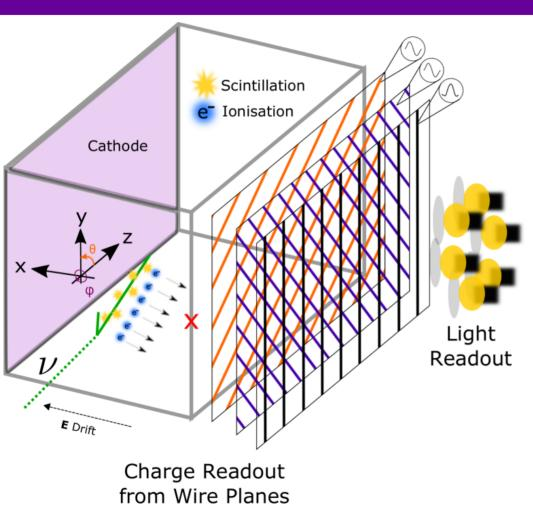
Scintillation and ionization signals used to produce bubble-chamber like images of events
