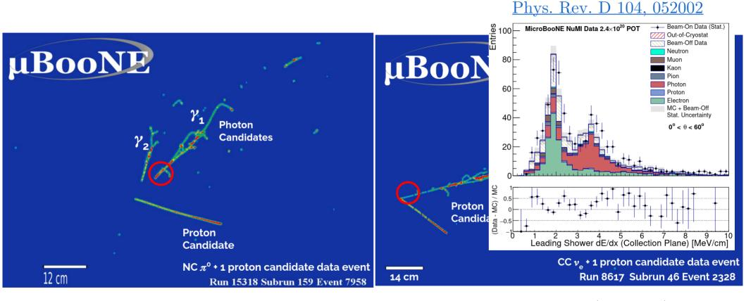
Starting segment of photon initiated shower has double the deposited charge  $(\gamma \to e^+e^-)$
