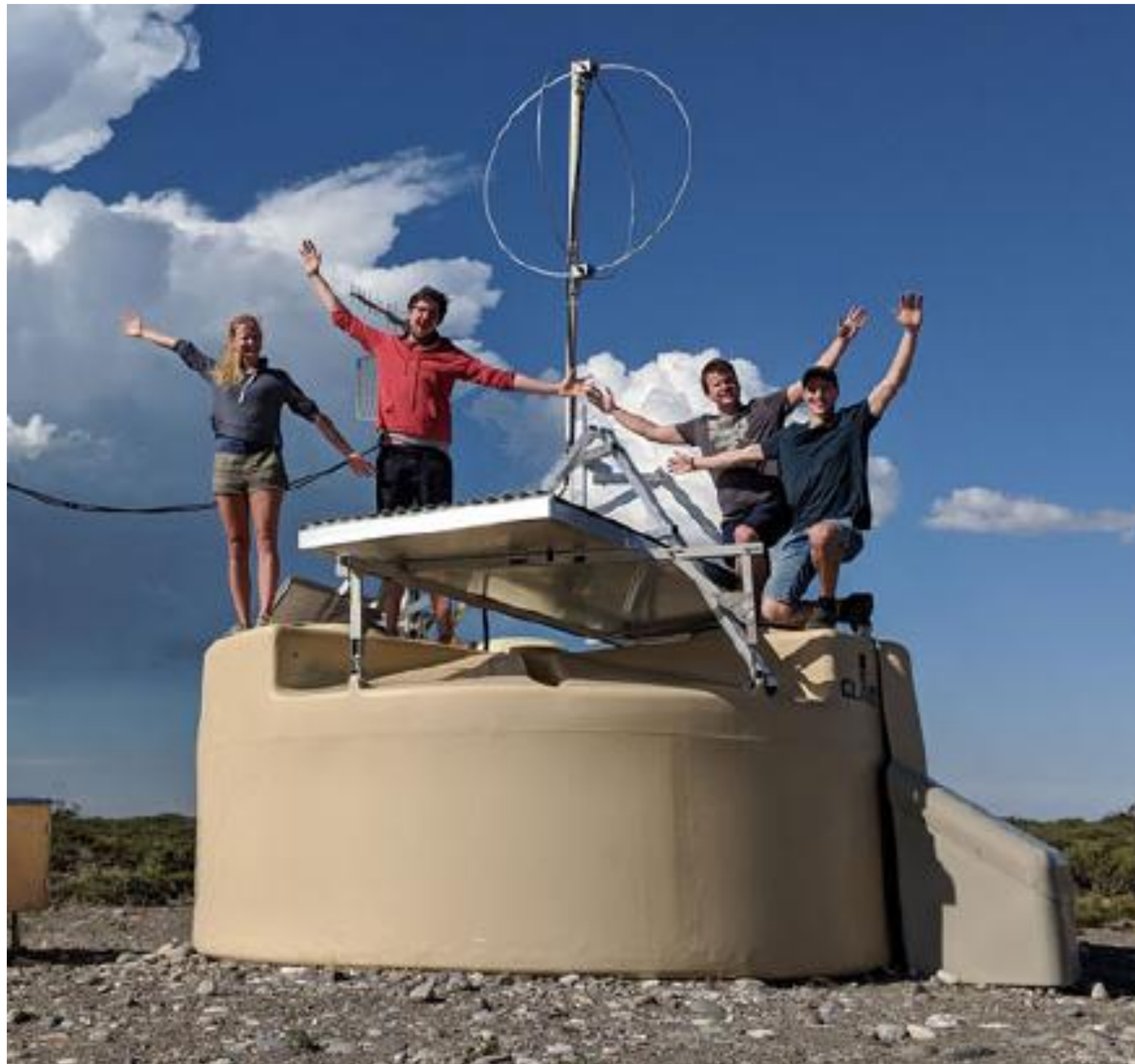
SD station with new scintillator and new radio antenna
