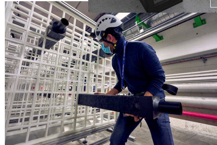
UA graduate student Aditya Upreti installing the MAPP's scintillators into the support structure, CERN, February 2022. (Image: CERN News )
