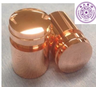
Regular flat cathode ~Φ20 mm, metallic
