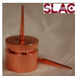
Pin-shape cathode ~Φ1 mm, metallic
