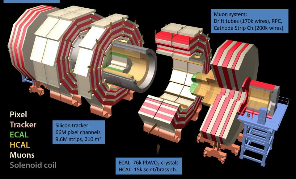
Total weight 12500 t, Overall diameter 15 m, Overall length 21.6 m, Magnetic field 4 Tesla
