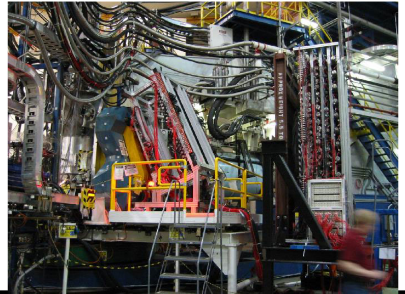
Test cell factor ~10 safety test, burst pressure above 3500 psi
