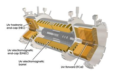
• Forward Calorimeter (FCAL) used to determine reaction plane
