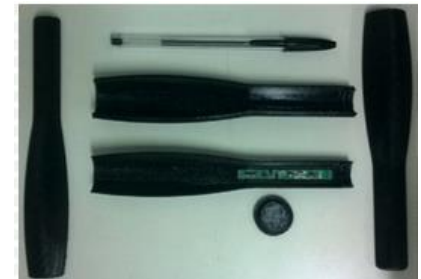
wireless probe for use in radio guided surgery
