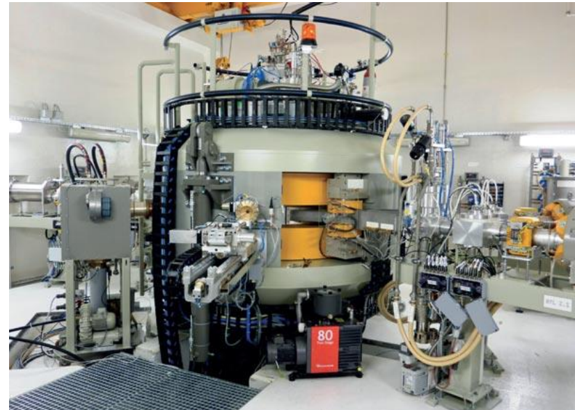
30 isotope-producing cyclotron with 2.7 m in diameter and 2.8 m high
