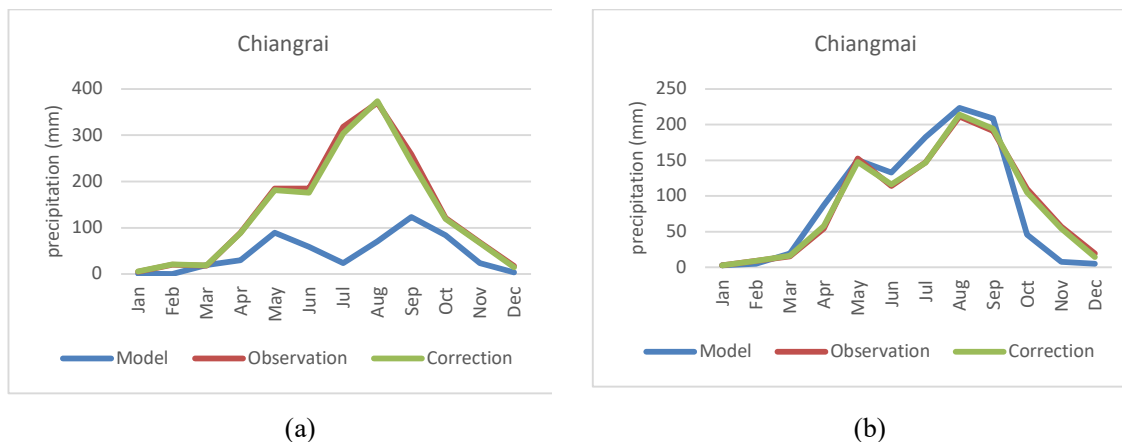
Figure 1. Averaged monthly simulated, observed, and corrected precipitation at (a) Chiang Rai and (b) Chiang Mai station during 1980-1999.
