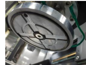
Gantry head with vacuum holes
