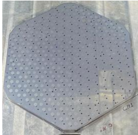
Low-density (LD) silicon sensor
