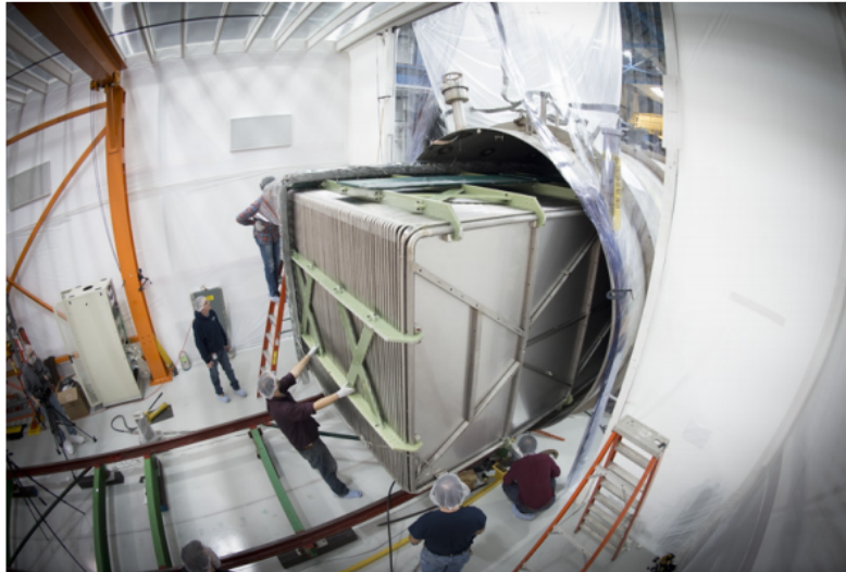
\mu booNE field cage being inserted into Cryostat (left)
