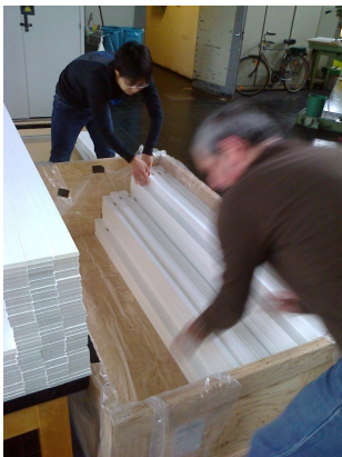
Extruded scintillator bars (1600 x 50 x 10 mm)
