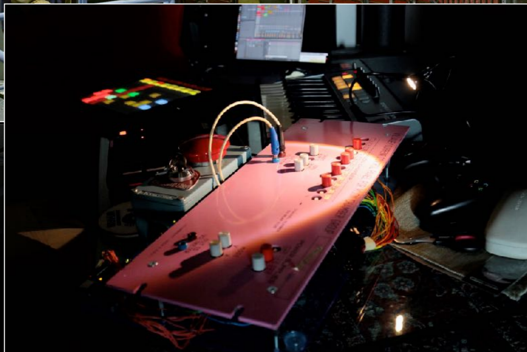
LV Control Panel for UA1 Muon System
