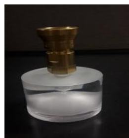
Collected Rn is transferred into a counter (Lucas cell)
