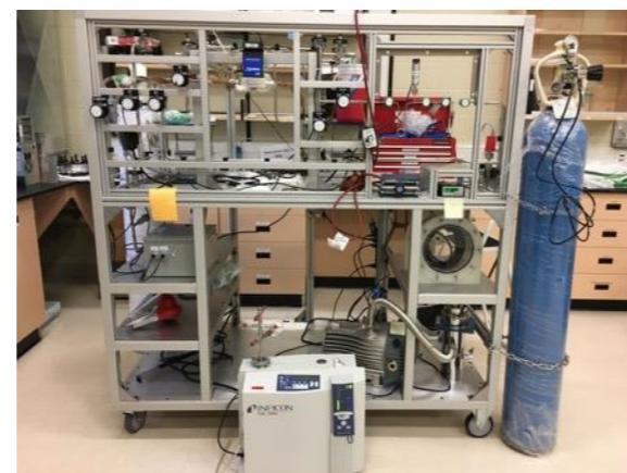
Perform Rn extraction using Rn gas board & allows most other residual gas to be exhausted from the system
