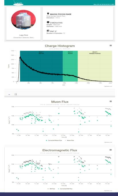
Data obtained on January 2018 during the Peruvian campaign at the Antarctic, the data is corrected by pressure.
