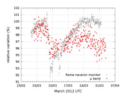
Results of Multi-Spectal Analysis of the Forbush Decrease of March 8th, 2012 measured in a single 1.8 m 2 WCD installed in Bariloche, Argentina (red stars), compared with measurements of the Rome neutron monitor (gray pluses), in two bands: EM-band (left), and  $\mu$ -band (right).
