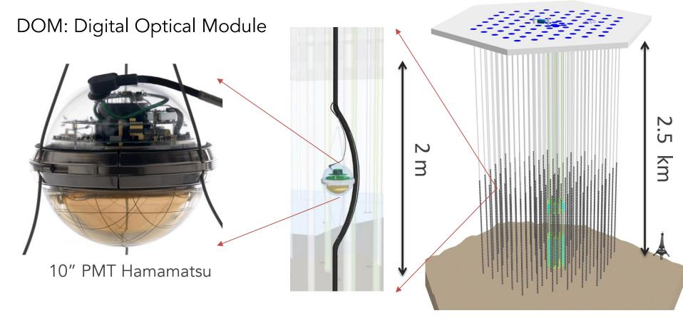
5160 DOMs spread over  $1 \text{ km}^3 = 1 \text{ Gigaton instrumented volume}$
