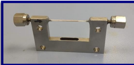
Reactor- \varnothing 1.5 mm X 2 cm catalyst bed - In situ X-ray techniques for characterization
