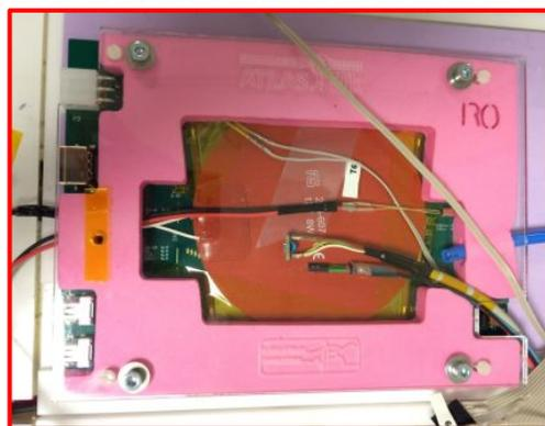
Module mock-up using heating pad
