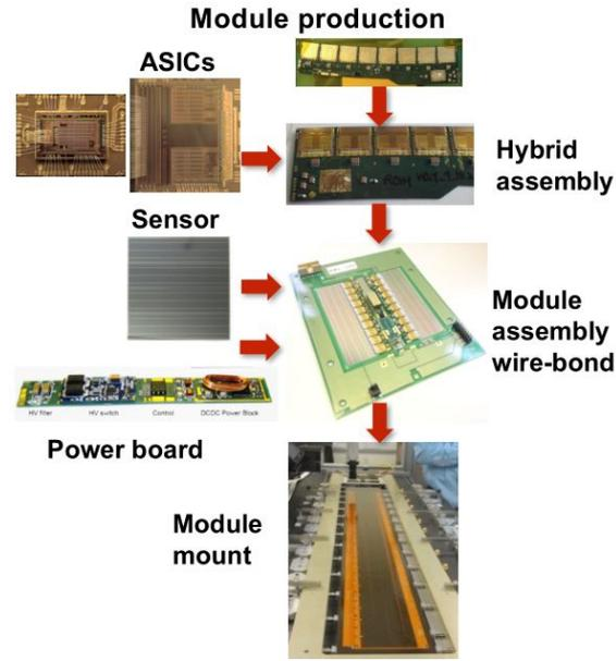
Production flow for barrel type modules, difference lies in sensor geometry.
