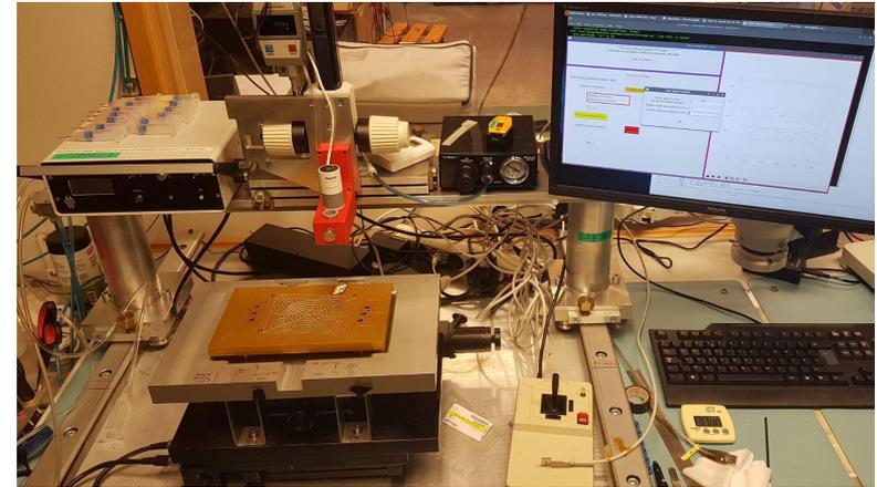
Gluerobot developed for hybrid-sensor assembly
