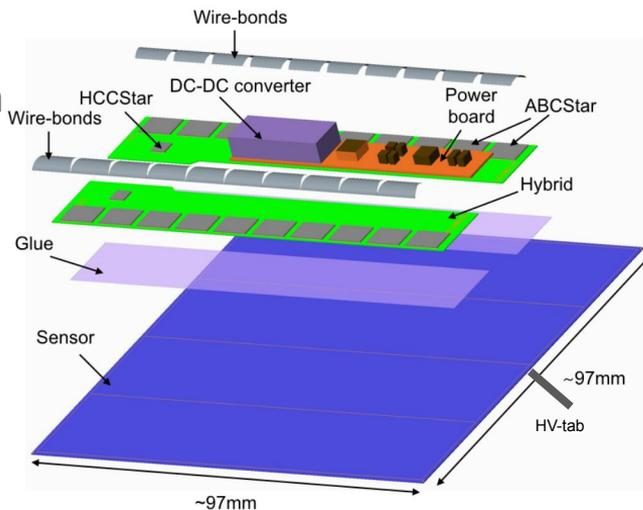
Exploded view of barrel type strip module
