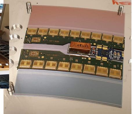
R0 module built as part of early prototyping. (front-end wirebonds missing.)
