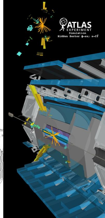
TileCal; after LAr cal is a segmented sampling calorimeter, steel plate absorbers and plastic scintillator tiles.
