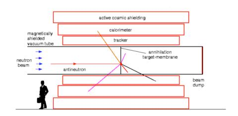
Residual B field <5 nT Residual vacuum < 10<sup>-5</sup> P
