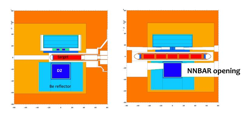
Monte Carlo Model of the ESS targer+moderator model fully parametrized to allow easy changes in the geometry for sensitivity studies and optimization.
