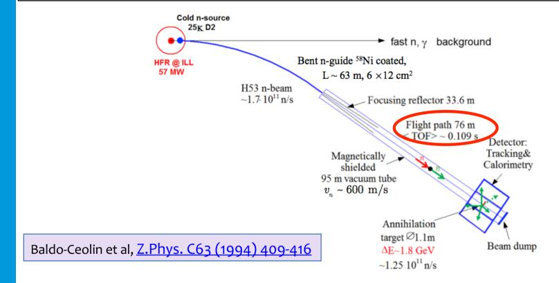
Nt<sup>2</sup> = 1.5 10<sup>9</sup>s, P < 1.6 10<sup>-18</sup> (run lasted ~1 year) and  $\tau_{n \to \bar{n}} > 0.86 \ 10^8$ s (N is the free neutron flux reaching the annihilation target and t is the neutron observation time).
