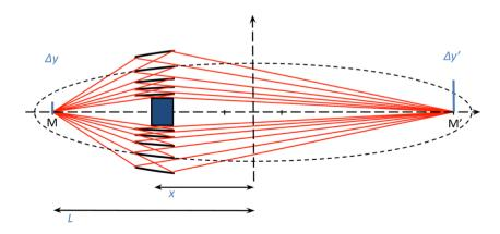
Much larger viewable area of the lower moderator -> optimised imaging instrument to extract a large divergence neutron flow and focus over long distance (~200m).
