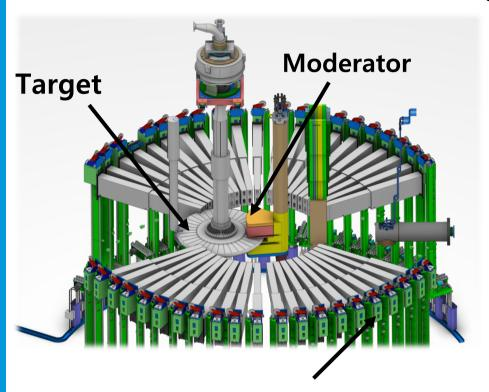
Neutrons are extracted from the target in the different beamport
