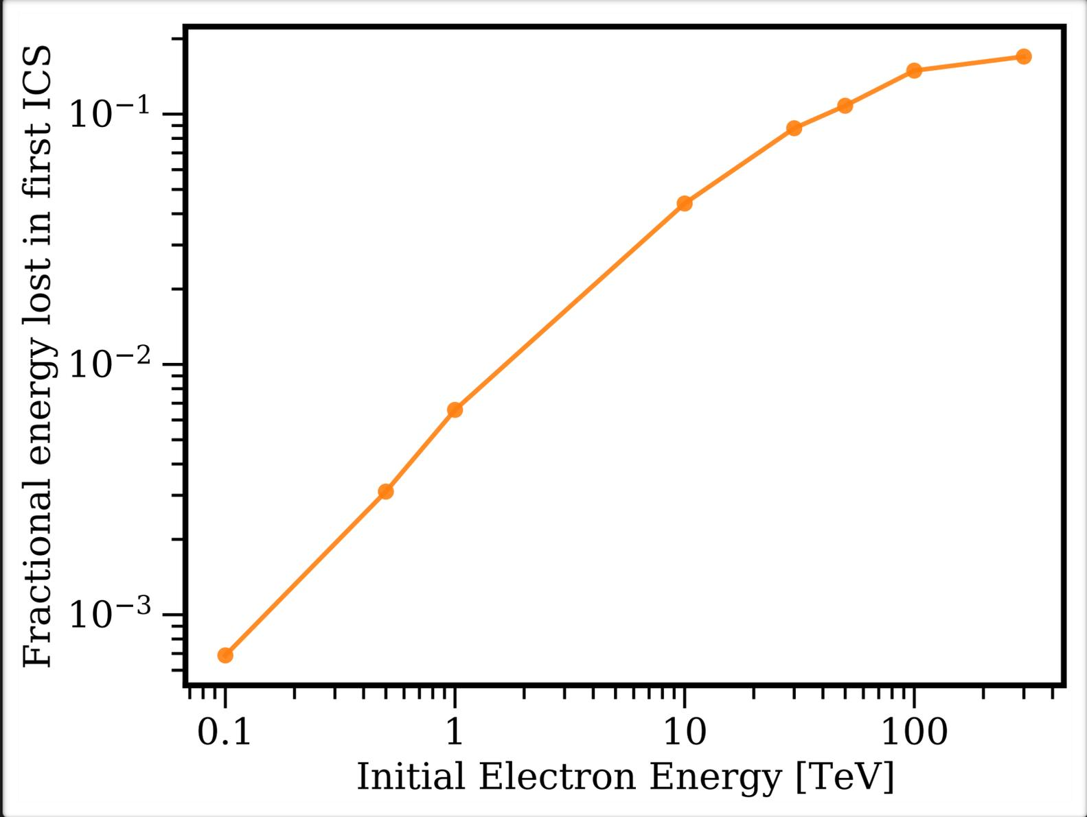
ICS interactions are rare, but take a large fraction of the energy in a single interaction, especially at high energies
