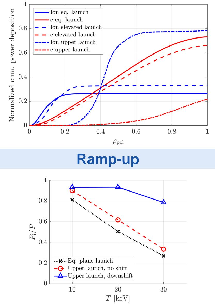
Upshift in  $k_{\parallel}$  yields high electron absorption, but lower CD efficiency [2]
