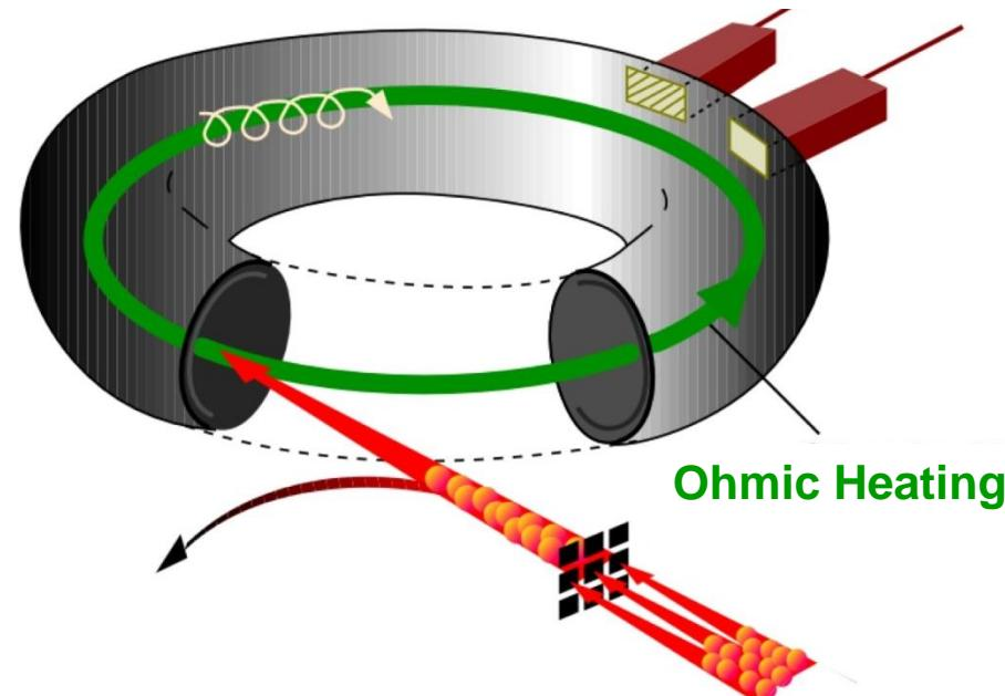
**NBI: 33 MW Neutral Beam Injection**
