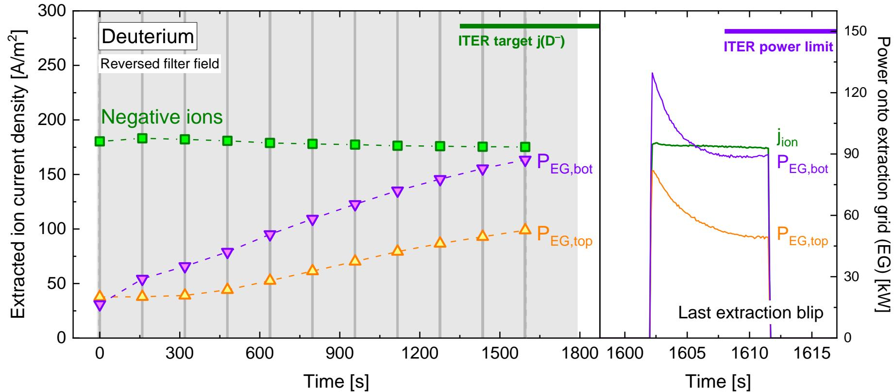
Stable ion current but strong temporal behavior and vertical asymmetry of co-extracted electrons
