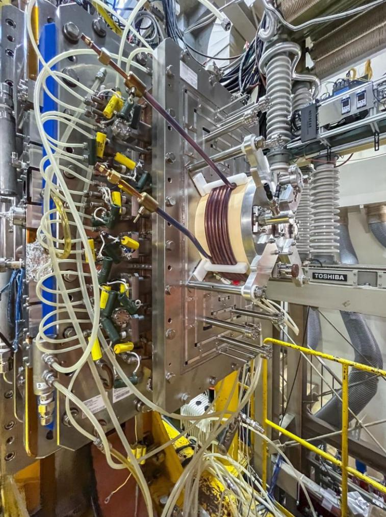
The RF ion source with the back plate attached to the NIFS NB Test Stand beamline – August 2022.
