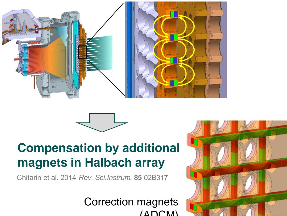
**Compensation by additional magnets in Halbach array**
