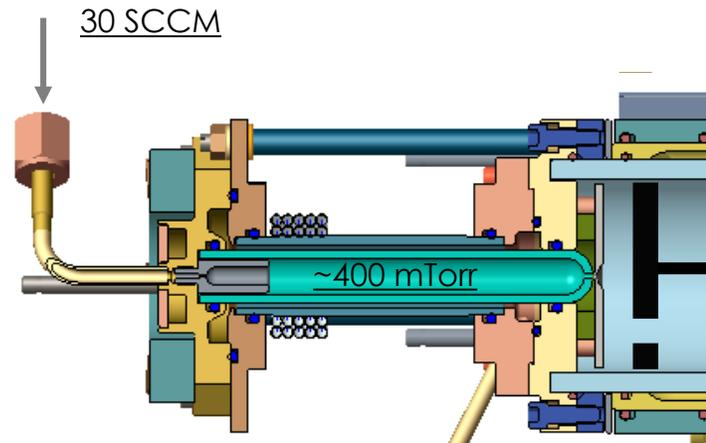
Collector electrode ~1 cm downstream of cathode
