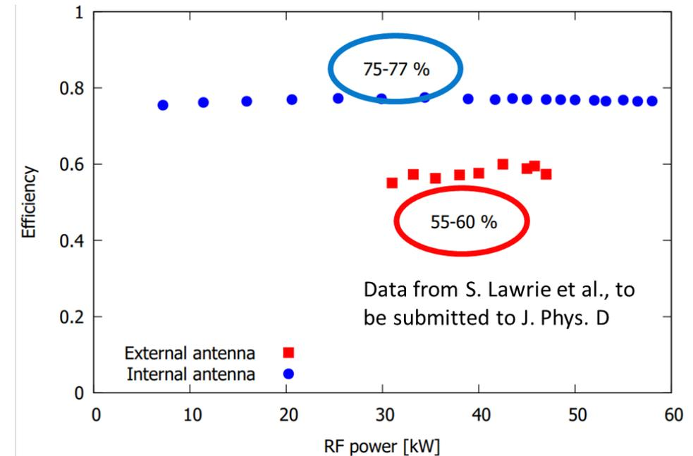
The internal antenna source has higher RF efficiency, almost 80%
