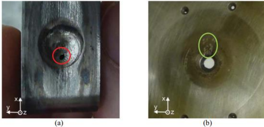
Figure 5. Wear traces on the (a) cathode and (b) the anode cover plate of BNL's magnetron. The location of the traces on the cathode and anode cover plate is indicated by a circle and an ellipse (red and green), respectively
