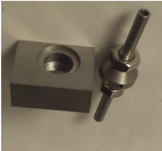
Fig. 2 Photograph of cathode and anode of modified magnetron SPS
