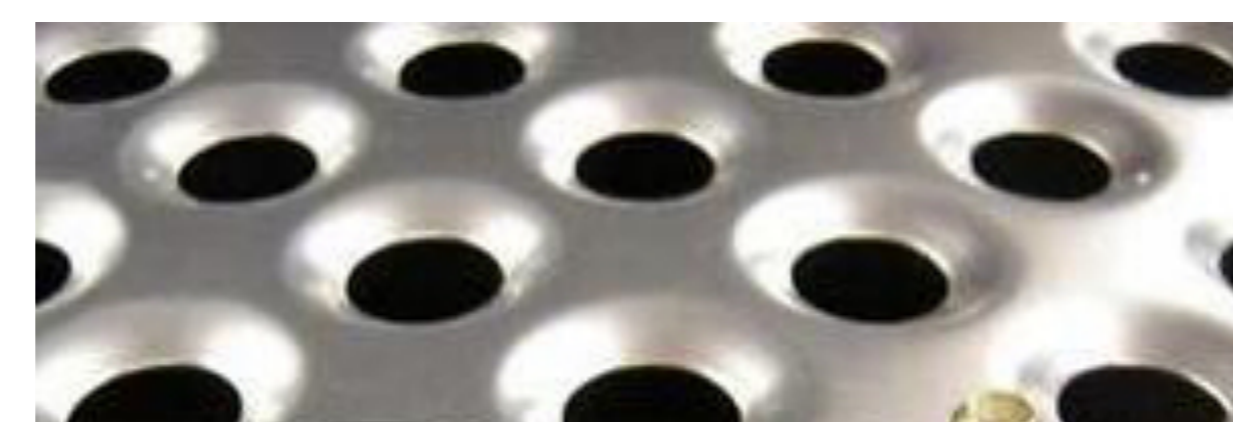
Fig. 5: example of bevelled aperture edges, considered for the reduction of the local electric field concentration at the aperture edges
