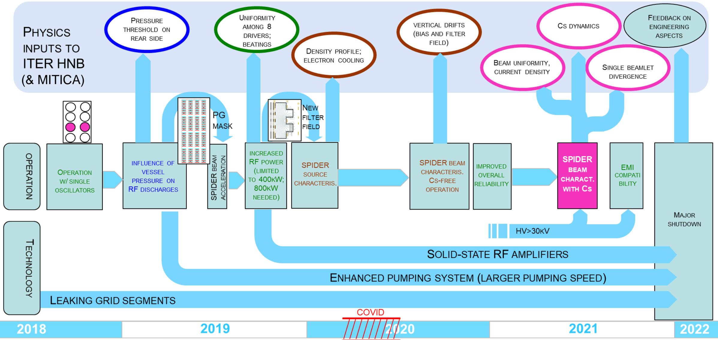
Among a large number of refurbishments and modifications, the core line of shutdown activities tackles the quest to the target SPIDER parameters (**uniformity**, **current density**, **divergence**), hence implying **full beam**, **high RF power** and **high voltage** with no discharges:
