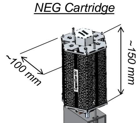
A preliminary assessment compared possible solutions (commercial cryopumps, custom cryopumps and NEG pumps), leading to the final choice
