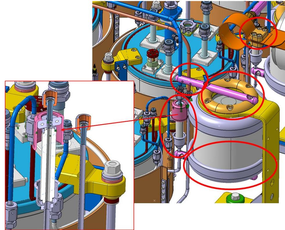
**RF driver modifications** (quartz case, stainless steel -copper coated RF coils, 1mm distance between RF coil and driver case, new coil support combs, EMSs electrically insulated from RDP) => **reduction of local E-field**
