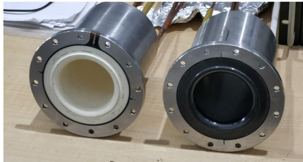
Al<sub>2</sub>O<sub>3</sub> (left) and Si<sub>3</sub>N<sub>4</sub> (right) plasma chambers for thermal and mechanical test
