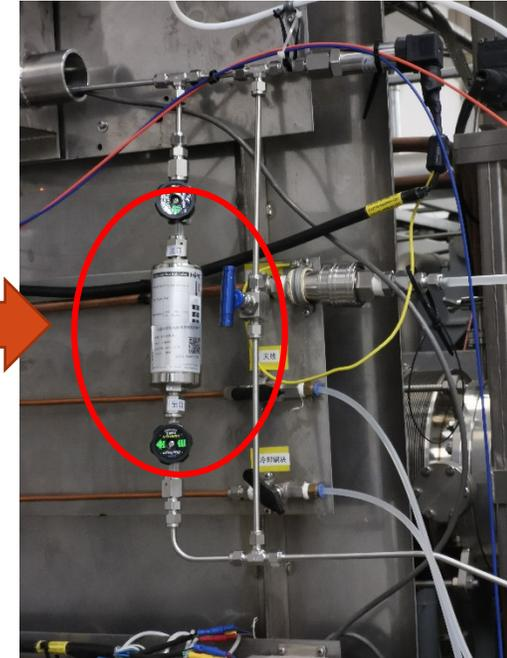
The hydrogen purifier eliminates the water/O<sub>2</sub> to less than 1 ppt according to the specification.
