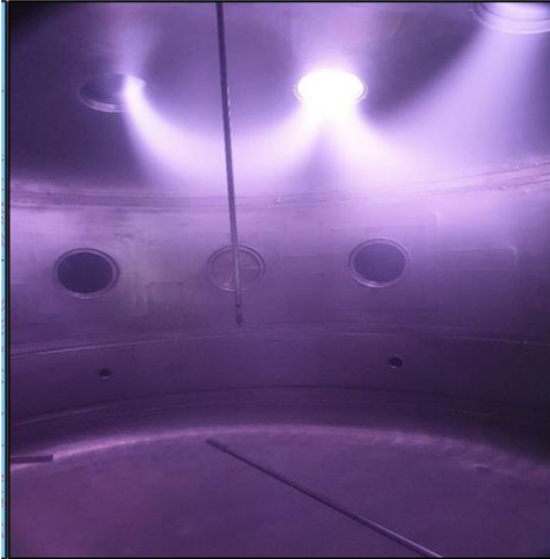
Plasma inside the chamber showing cusp configuration
