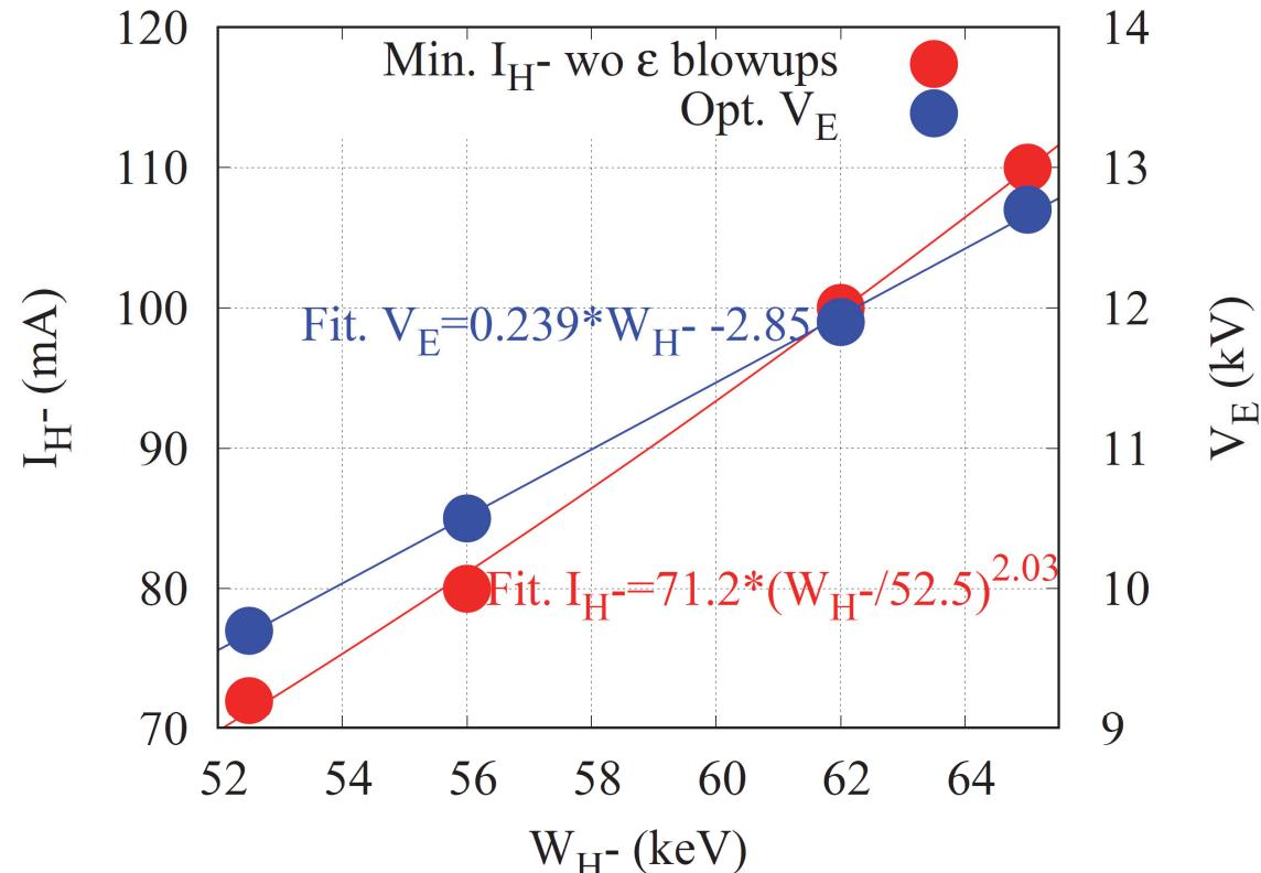
Measured relationships between  $W_{H^-}$  &  $I_{H^-}$  without any emittance blowups,  $W_{H^-}$  & optimum  $V_E$  plotted with red closed circles and blue closed circles, respectively. Fitted  $I_{H^-}$  &  $V_E$  equations are shown with red & blue lines, respectively. Square (not 3/2 power) dependence of  $I_{H^-}$  on required  $W_{H^-}$  is essential for next IS & RFQ design.
