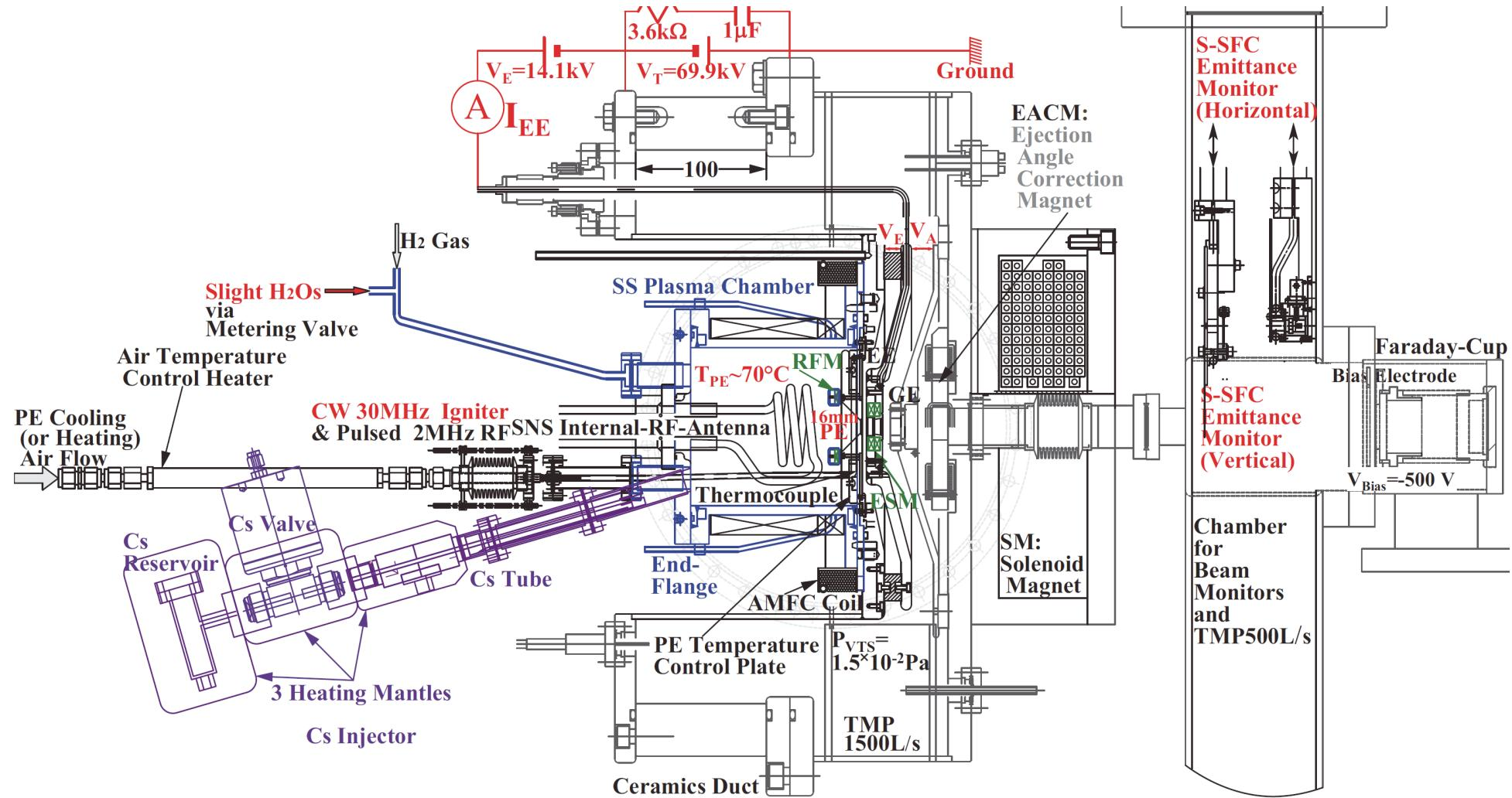
High  $I_{H^-}$  & Brightness & RF power efficiency by Thick PE(16mm-45°:  $1.5I_{H^-}$ ) , Slight H<sub>2</sub>Os Feeding( $0.5\varepsilon_{nrsmx/y}$ ), Low  $T_{PE} \sim 70^\circ C$ ( $0.75\varepsilon_{nrmsx/y}$ ), CW-30MHzRF igniter( $1.2I_{H^-}$ : 17SCCM for  $\phi_{PE} = 9\text{mm}$ ): 94.3% RFQ accl. effi. for 72mA, ( $I_{H^-}$ ,  $W_{H^-}$ ,  $V_E$ , duty factor) = (110mA, 66.6keV, 13.4kV, 4.5%)@NIBS2020  $\Rightarrow$  (120mA, 69.9keV, 14.1kV, 4%)
