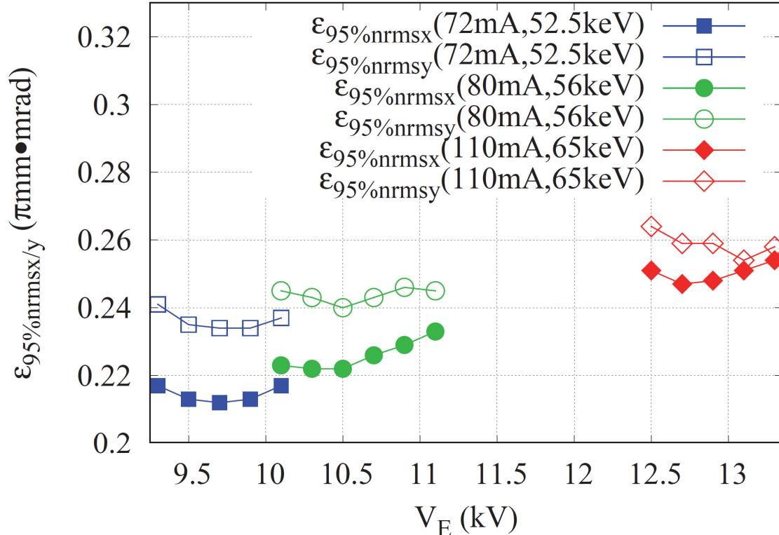
Measured relationships between  $V_E$  and  $\varepsilon_{95\%nrmsx/y}$  for conditions of  $(W_{H^-}, I_{H^-}) = (52.5 \text{ keV}, 72 \text{ mA})$ ,  $(56 \text{ keV}, 80 \text{ mA})$  and  $(65 \text{ keV}, 110 \text{ mA})$ , plotted with blue open or closed squares, green open or closed circles and red open or closed diamonds, respectively.
