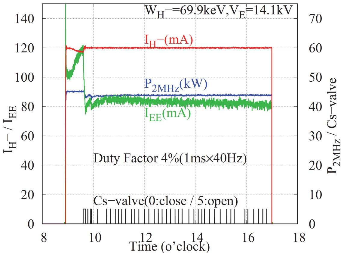
Trend graph of  $I_{H^-}$ ,  $I_{EE}$ ,  $P_{2MHz}$  and Cs-valve close/open during 8 hours operation, in which  $I_{H^-}$ , was feedbacked to  $120 \pm 1 \text{ mA}$  by  $P_{2MHz}$ , for  $W_{H^-}$  and  $V_E$  of  $69.9 \text{ keV}$  and  $14.1 \text{ kV}$  (pow. sup. max), respectively. In station. state, Cs inject. rate =  $42.3 \mu\text{g}/\text{hour}$ .
